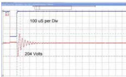
In air, there is no conductivity between the electrodes. The output signal waveform appears as shown.
